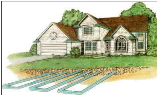
DIAGRAM OF GEOTHERMAL HVAC SYSTEM
