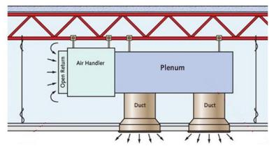
tions below the floor in places such as data centers. If there was ever a fire within the plenum, the air handler could assist in causing rapid fire development, similar to how we use our fans or our mouths to move air across hot coals or kindling to stoke a fire. Due to this concern, the code restricts what materials are permitted within air plenums. The International Mechanical Code reads as follows:
