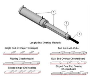
Tested Plenum Wrap Assembly - EXAMPLE ONLY
